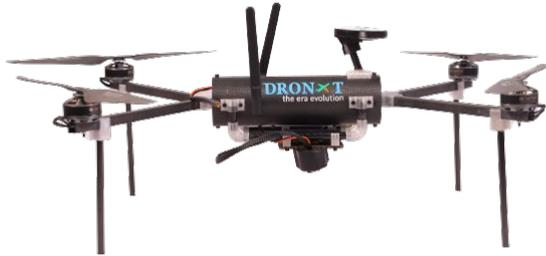
Rodnxt-S6, the first flagship multirotor UAV developed by Dronxt for surveillance missions delivers a strong 40 mins of operational endurance in a completely loaded configuration. With an innovative monocoque rugged airframe structure, it holds up heavily against adverse weather and terrain conditions.
